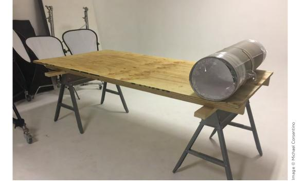
I built a DIY product-photography worktable using two sheets of 4x8 plywood, 2x4's and a pair of collapsible sawhorses. This can be easily stored when not in use.
